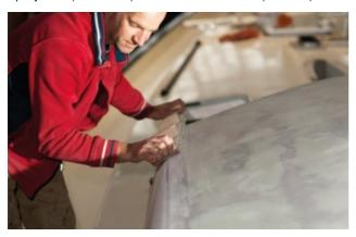
degrease and sand with 60-80 dry abrasive paper to a smooth surface.
